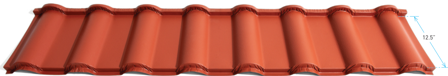
PVDF PRE-PAINTED GALVALUME (AZ 165) STEEL SYSTEM WITH KYNAR 500 ® RESIN ASTM-A792 SS GRADE "33" GAUGE: 29 (.017" THICK)
